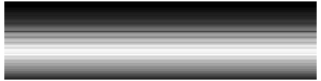
FIGURE 17. Spectral scan of the image of a homogeneous white test object after the calibration procedure with coefficients l_k(j) (without approximation) (before calibration see Figure 7).
