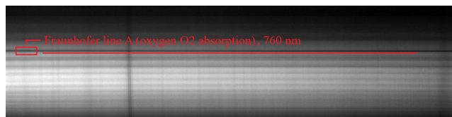
FIGURE 7. Spectral unfolding of the image of a white object illuminated by sunlight.
